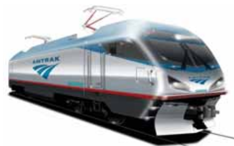
Amtrak Rendering of the recently ordered Amtrak Citie Sprinter ACS-64 electric locomotive from Siemens.
